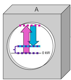
**A:** Customer load is greater than the power generated, so the net usage is positive. The meter will count forward based on the net usage.
