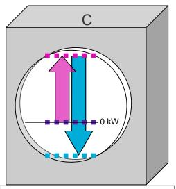
**C:** Customer load is less than the power generated, so the excess power is exported onto the grid. The meter will remain still.
