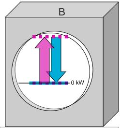
**B:** Customer load is equal to the power generated, so the net usage is zero. The meter will remain still.
