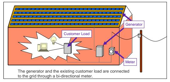
At the end of the billing cycle, the meter is read to determine how much it has counted forward. Then, the customer will be billed at their normal rate (\$/kWh) multiplied by how many kWh the meter has counted during the billing cycle.
