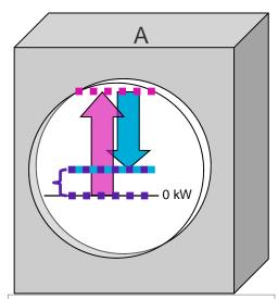
**A:** Customer load is greater than the power generated, so the net usage is positive. The meter will count forward based on the net usage.
